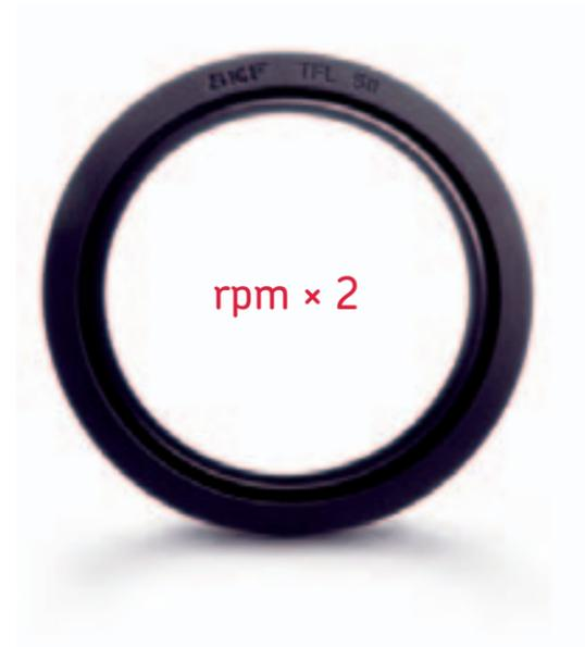
*A modern double-lip low friction seal hydrogenated nitrile butadiene rubber (HNBR) keeps lubrication in position and shuts out contaminants. The new solution allows rotation speed limits twice that possible with traditional felt seals.*
