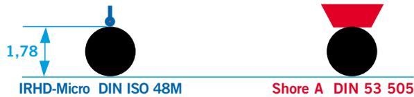
The IRHD is measuring on a 2 mm sheet during 30 seconds. The Shore A is measured on a 6 mm sheet during 3 seconds. The first method is very sensitive for surface imperfections. The second method is difficult for measuring at small cross-sections.
